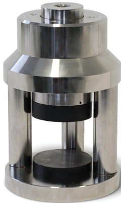
Compression device to test 50mm (2") cubes (50-C9032/H)
